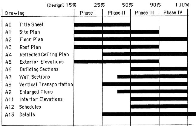
Fig. 1. Phase development of typical construction drawings indicate evolution of the documents
